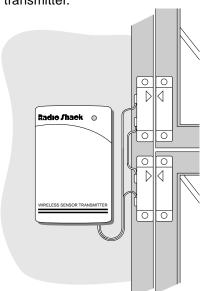
You cannot use NO (Normally Open) magnetic switches with this sensor transmitter.
